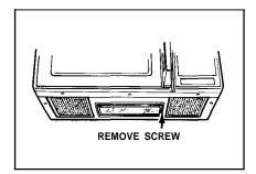
To replace combination cooktop light/night light, first disconnect **power** at main fuse or circuit **breaker panel or pull plug.**Remove screw on right side of light compartment cover and lower cover until it stops.
